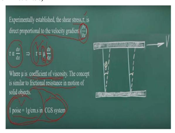
And shear stress will develop at this interfaces level and many of the studies the experimentally establish that this shear stress will have a directly proportional to the velocity gradient okay. If the more the they have the directly proportionality okay. That means more the velocity gradients is there so we will have the more shear stress. But it has a directly proportionality quantity.
