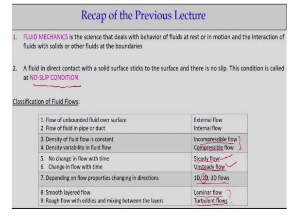
In fluid mechanics as you discussed is that we are talking about the behavior of the fluid either at the rest or in the motions and also the interaction of fluids with the solids or other fluids at the boundary. The more important concept what we have discussed is no-slip conditions. That means, when a fluid is moving fluid in a stick with a solid surface, the velocity of the moving fluid is equal to the velocity of the solid surface. That is what at that point the no-slip conditions exists.
