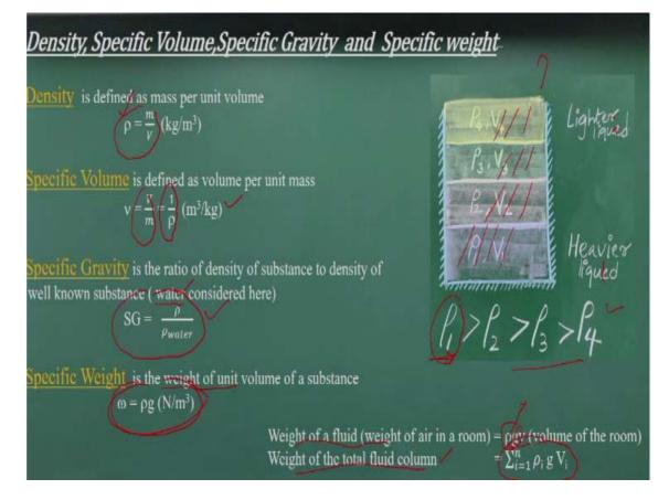
That is the reason as I told earlier that if I consider a small volume of the fluid the mass of the fluid if I measure it okay, as the volume of the sample in volume is larger than the limiting volumes for the continuum hypothesis. So if I consider that part and get a mass of that fluid and do a mass per unit volume. That means we are that is what is the density:
