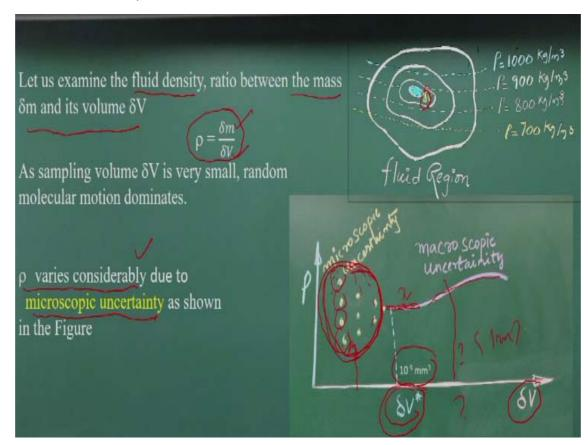
So these properties what is happening it at the molecules levels that is what is reflect us very interesting concept what let us consider very basic fluid properties is the fluid density, okay? That means that is what is the mass per unit volumes. That means, if I consider a very tiny  $\delta V$  and that  $\delta V$  is the sample volume for me. And if I consider that sample volumes, I will have the density the  $\delta m$  by  $\delta V$ , okay, mass per unit volume.
